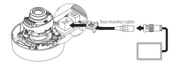
2. Adjust the zoom and focus. Adjust the Pan/Tilt/Rotation position of the camera.
