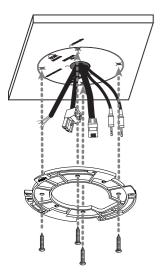
3. Connect the cables to the cable jacks of the camera body.
