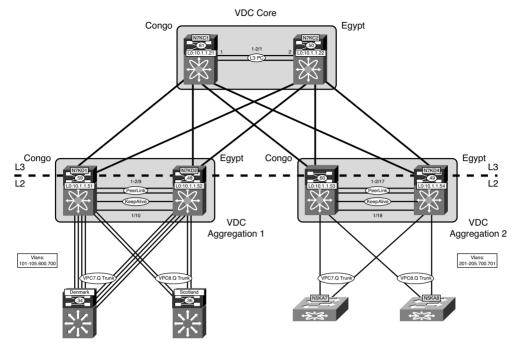
Figure 1-5 Logical Segmentation with VDCs on the Nexus 7000
