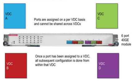
Figure 1-23 N7K-M206QF-23L I/O Module Interface Allocation
