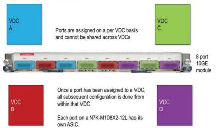
Figure 1-19 N7K-M108X2-12L Module Interface Allocation
