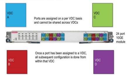
Figure 1-22 N7K-M224XP-23L I/O Module Interface Allocation
