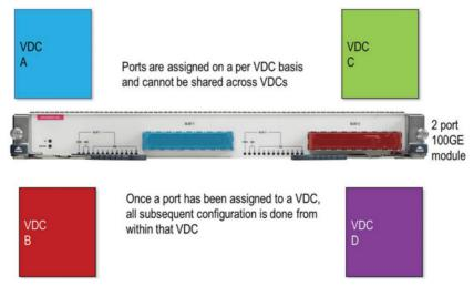
Figure 1-24 N7K-M202CF-22L I/O Module Interface Allocation
