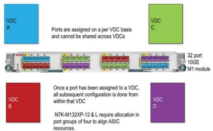
Figure 1-17 N7K-M132XP-12 and L Module Interface Allocation
