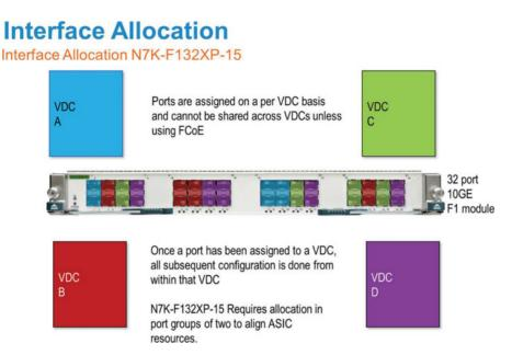
Figure 1-18 N7K-F132XP-15 Module Interface Allocation
