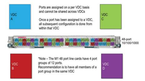
**Figure 1-20** N7K-M148GS-11 and L Module, N7K-M148GT-11 and L Module Interface Allocation
