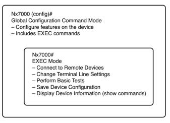
Figure 1-1 NX-OS Command Access from EXEC Mode to Global Configuration Mode
