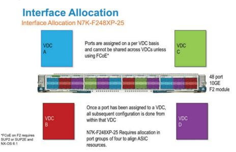
Figure 1-21 N7K-F248XP-25 I/O Modules Interface Allocation
